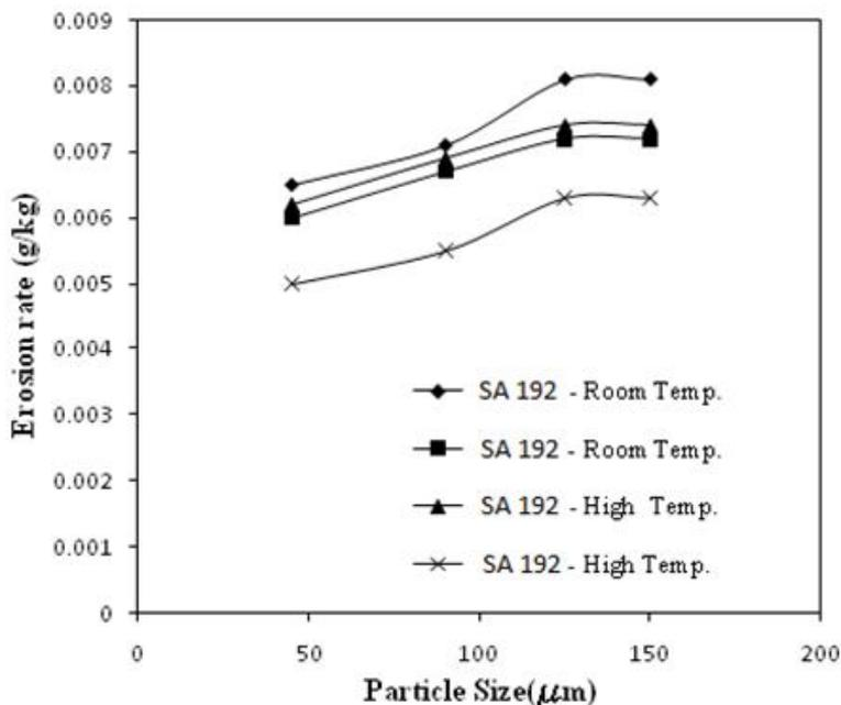
Figure 5: Effect of fly ash particles size on tube erosion SA-192 (SH&SC)
