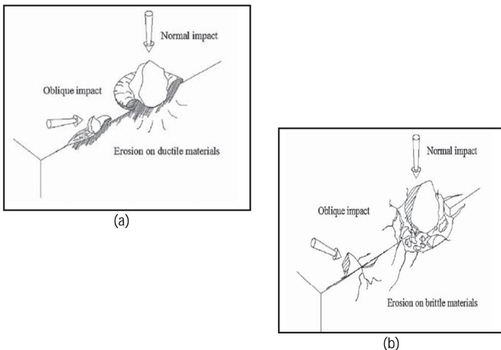
**Fig. 1 (a) & (b): Erosion mechanisms in ductile and brittle material**
