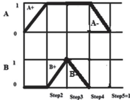
Figure 3: Functional Diagram
