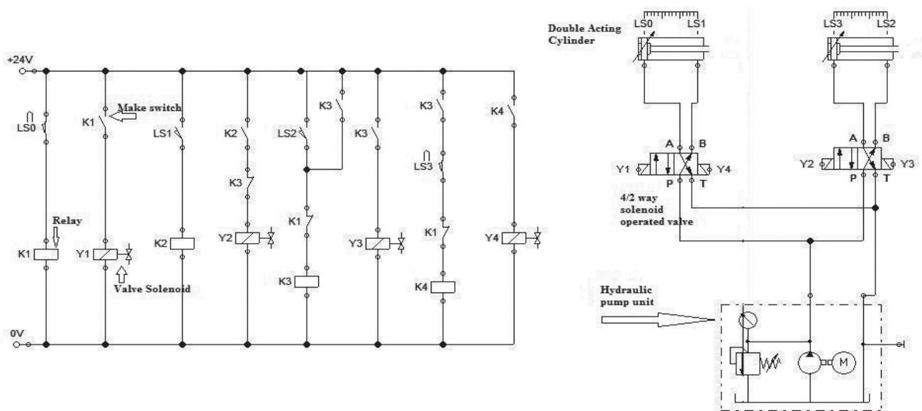
Figure 4: Electro-Hydraulic Circuit
