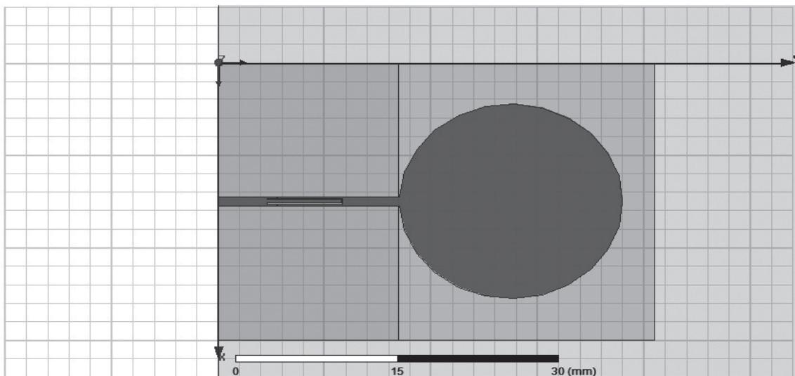
**Figure 1: Circular Patch with BPF and Result**
