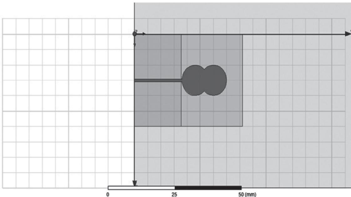
Figure 6: Top view of dumb bell shaped Patch (vertical)
